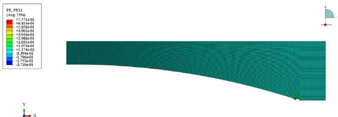
Figure 58 - Plastic deformation associated with a plane stress-strain thickness of 3 mm.
