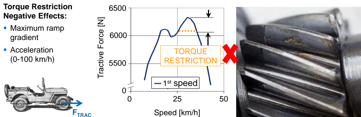
Figure 2.2 – Longitudinal dynamics analysis and the projection of the torque restriction over the 1st speed regime (REGO, 2011).
