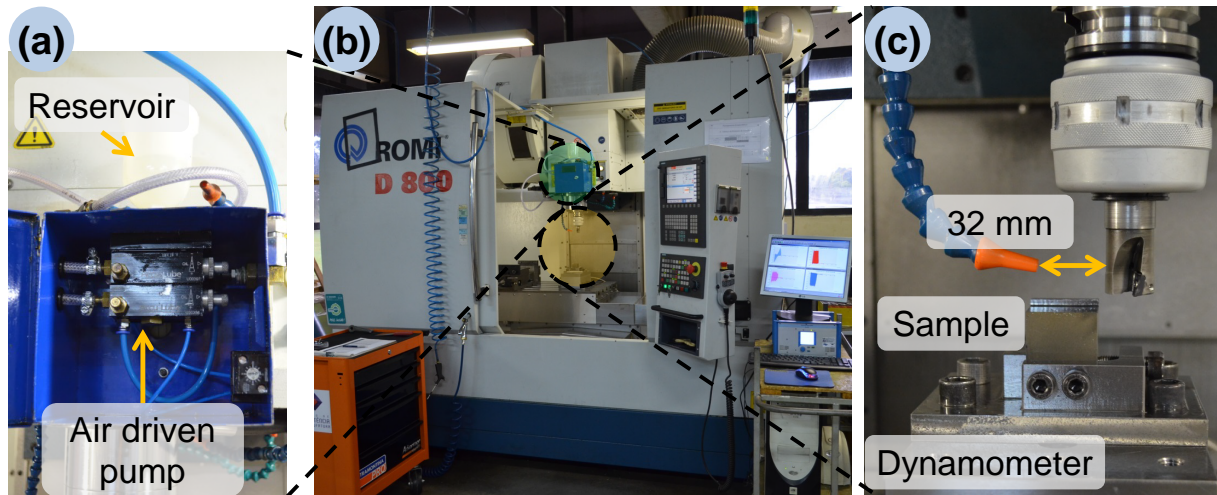
Figure 4.6. Experimental setup for the machining experiments. (a) Accu-Lube MQL equipment; (b) machine tool with the MQL device and dynamometer installed; (c) close view of the tool, MQL nozzle, sample and its support over the dynamometer.
