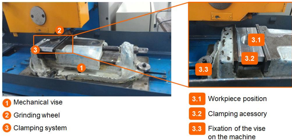
Figure 4.9 - Description of the grinding process used for the cylindrical workpieces.
