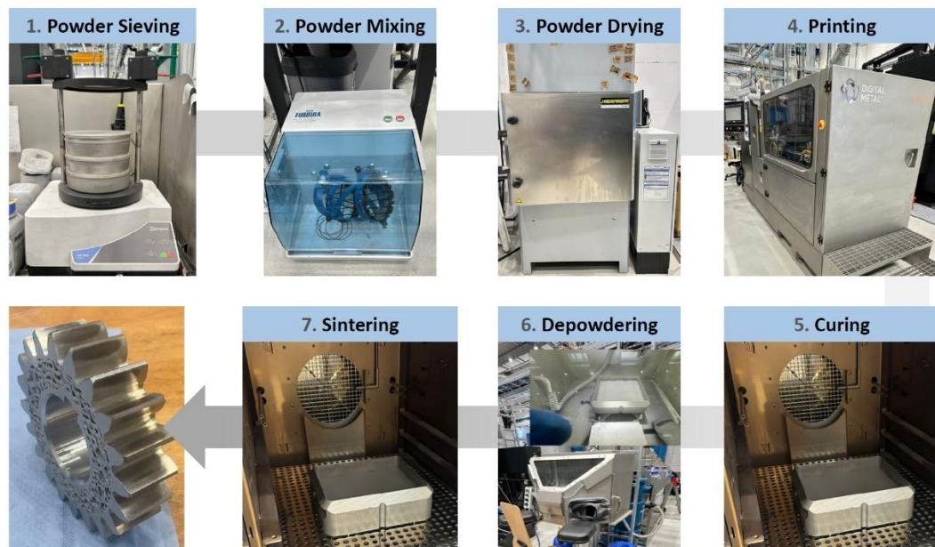
Figure 2-5: Binder Jetting process steps: powder preparation (sieving, mixing, drying), layer-by-layer printing with binder, thermal curing, depowdering, and final sintering. Each step directly influences the final part's density and integrity.
