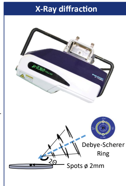
Figure 4-8: Residual stress assessment procedure
